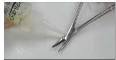
We can't notice rust if the rust has been caused inside a joint. Rust spreads gradually and suddenly breaks a part in two parts someday. Please do oiling before sterilization. Oiling every time before sterilization is the best way to keep your instruments live long.
