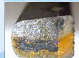
Long-term storage also can be the cause of rust due to the storage conditions. Not only doing cleaning and drying properly but also oiling to a joint part are required. These processes can prevent rust and keep instruments moving smoothly. And please unlock a ratchet and open a joint part during sterilization.
