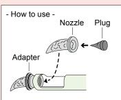
\*Resin of necessary quantity is filled in a nozzle, and a plug is inserted in and it is used by equipping into
